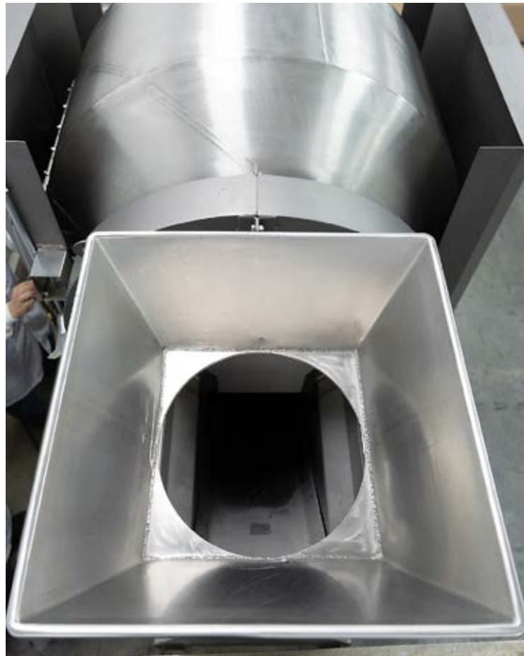
The Rotary Batch Mixer loads, blends, and discharges from a stationary outlet in about 15 minutes.
